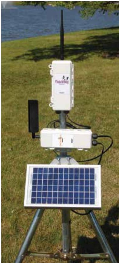
3923 DataScout cellular Modem mounted with a WatchDog Retriever
